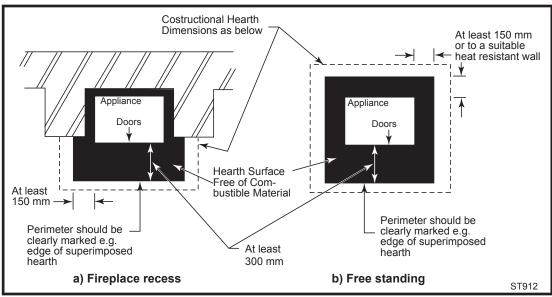
Fig. 10 Noncombustible hearth surface dimensions.
